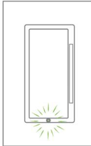
Once power is restored, the status LED will blink GREEN indicating your device is in setup mode. See page 15 if your Status LED is not blinking GREEN.
