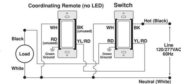
**NOTE:** The switch must be installed in a wall box that has a Line Hot and Neutral connection. The coordinating remote must be installed in a wall box with a Load connection and a Neutral connection. A Neutral wire to the coordinating remote needs to be added as shown. If you are unsure about any part of these instructions, consult an electrician.
