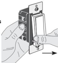
Insert top tabs and press in bottom tabs to attach
