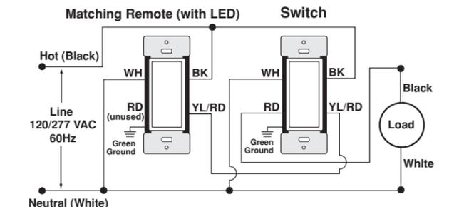
**NOTE:** The switch **must** be installed in a wall box that has a Load and Neutral connection. The matching remote must be installed in a wall box with a Line Hot connection and a Neutral connection. A Neutral wire to the matching remote needs to be connected as shown. If you are unsure about any part of these instructions, consult an electrician.
