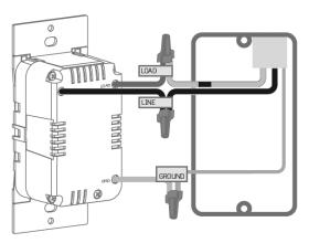
**Note:** Line, Load and Ground connections are required for proper operation.
