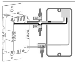
**Note:** Line, Load and Ground connections are required for proper operation.
